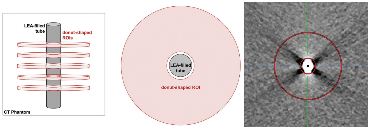
FIG 1. Schematic illustration of the donut-shaped ROI created by the MITK with an inner radius of 6 mm and an outer radius of 26 mm. The tube filled with the LEA of interest was placed centrally with a radius equal to the radius of the donut hole. For each tube, the measurement was performed with an ROI in 5 different positions according to the length of the LEA cast.
