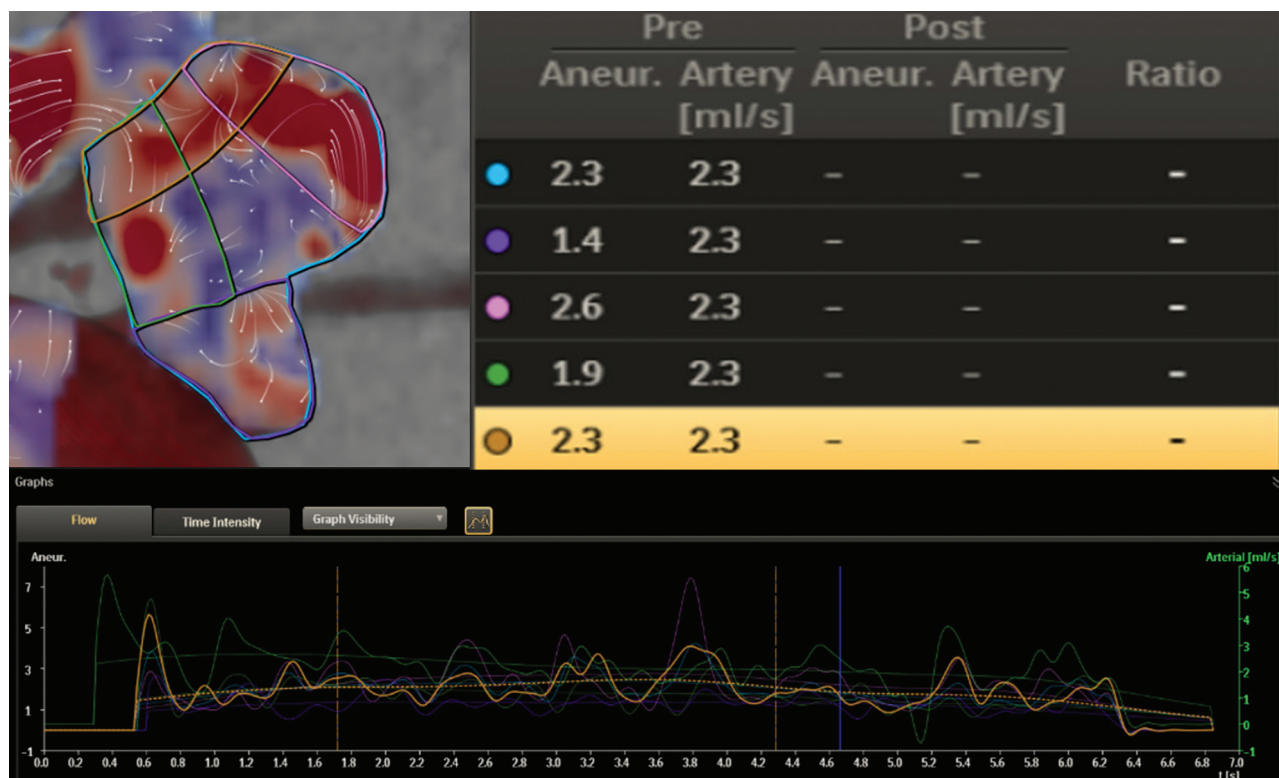
FIG 3. Measurement of MAFA of the daughter sac of the aneurysm on the AneurysmFlow Tool. Measurement of the MAFA of the entire aneurysm (ROIs in turquoise). Measurement of the MAFA of the daughter sac of the aneurysm (ROIs in violet). Measurement of the MAFA of the inflow region of the aneurysm (ROIs in pink). Measurement of the MAFA of the neck region of the aneurysm (ROIs in light brown). Measurement of the MAFA of the outflow region of the aneurysm (ROIs in bright green).
