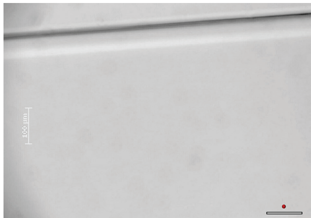
Fig 4. Freeze frame from On-line Video 5 of DSP flowing through a 200- \mu m-depth channel after mixing with LA and plasma. The straight line at the top of the image is the edge of the channel. No crystals or significant particulates are identified. The white scale bar in the bottom right of the image represents 100 \mu m. The adjacent red circle represents the average size of a RBC at this magnification. There is a separate scale bar on the left side of the image.
