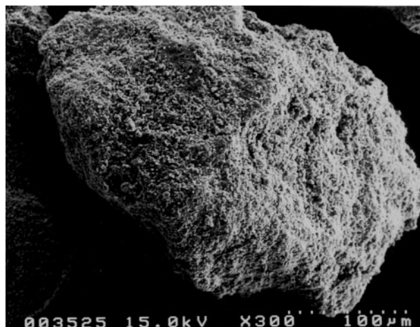
FIG 1. Scanning electron microscopic image shows the oval shape of hydroxyapatite ceramic microparticles. Surface has microporous structure with no spine (original magnification, \times 300 ).
