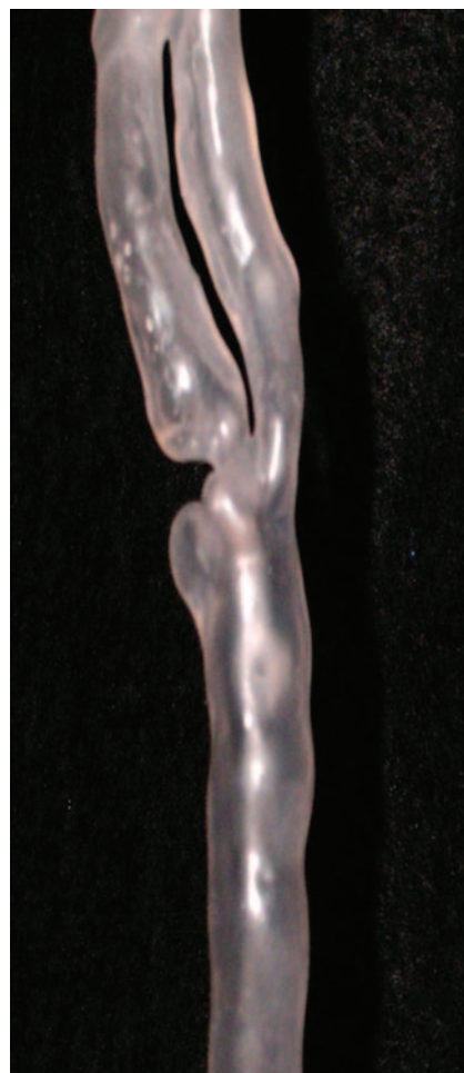
FIG 3. Silicon replica made by the lost-wax technique. This replica was then used to study the flow dynamics of this patient by placing it in a neck phantom and perfusing non-Newtonian fluids while injecting isobaric dyes into the slipstreams (not shown here). The replica was next placed into the scanner, the fluid in the phantom was made isoattenuated to the silicon with contrast agent, and the entire phantom was scanned by using the same scan parameters as were used to scan the patient.
